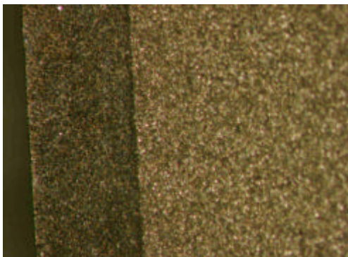
Figure 13: EDM polished edge
