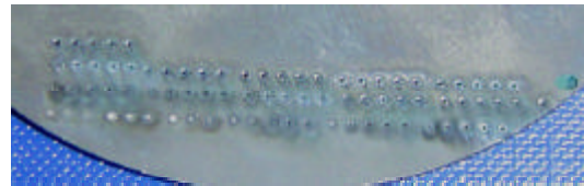
Figure 8: Pierce-through test matrix with air assist gas.
